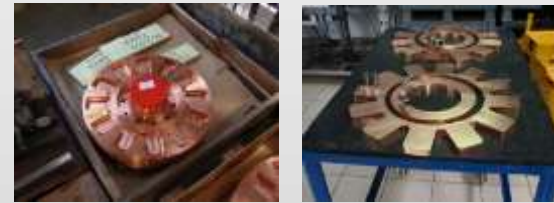
SDMS parts of end discs ready for e-beam welding
