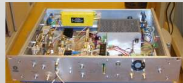
IQ modulator / demodulator LLRF rack [ESRF project leader: G. Gautier]
