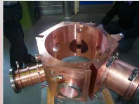
SDMS: Body after e-beam assembly of the 3 sectors, November 2010
